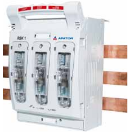
RBK 1-SG*(top cable terminal) RBK 1-SD*(bottom cable terminal) for installation on to 60 mm busbar system top/bottom cable terminals: - M10 screw terminals - S-bridge clamps - V-shaped terminals
