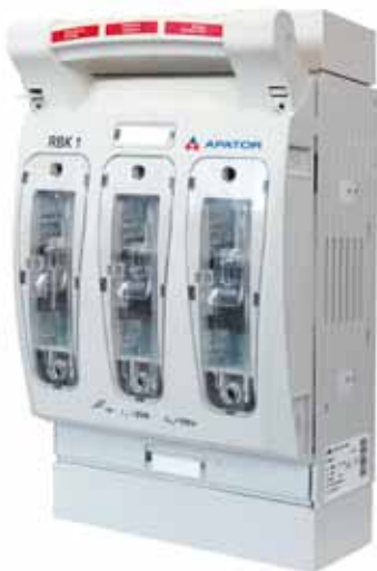
RBK 1 pro - O for installation on mounting plate with additional cable terminal shrouds cable terminals: - M10 screw terminals - S-bridge clamps - V-shaped terminals
