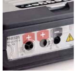
Shutter to prevent hazardous lead combinations.
