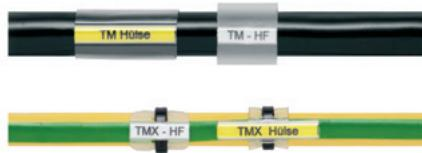
The range of TM sleeves is comprehensive and permits almost universal use: from thin conductors to cables with a large outside diameter, a wide range of applications is covered. The sleeves protect the printed inlay tags against external influences. TM sleeves also permit flexible installation. They are available in five different lengths (12, 15, 18, 20, 30 mm) and 11 sizes – one tag type for all sleeves.
