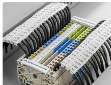
SFM: The wire markers have an open design and can be easily and quickly installed before or after the wiring process
