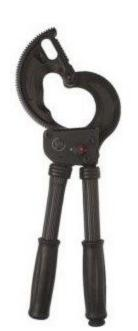
Very solid and easy to use reinforced cable cutter, with a wide range of applications. Blades made out of chrome - nickel steel. Reliable, well proven, needle-roller bearing ratchet drive. All steel parts are hardened. Quick blade release allows fast backout in any position. This cable cutter separates also cable with thin sheeting. Can be used even in confined areas.
