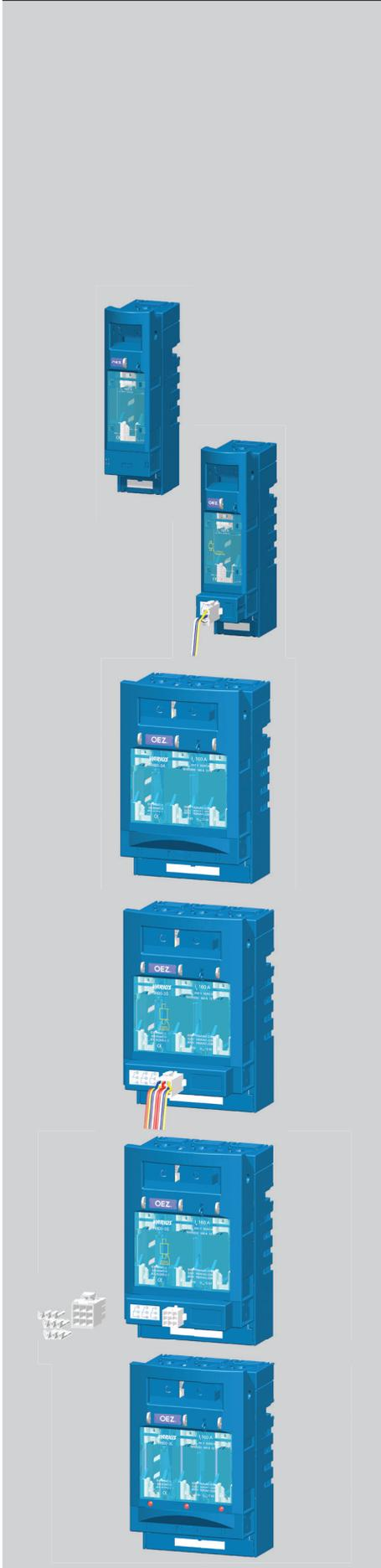
Fuse switch-disconnector FH00 is intended fuse-links with blade contacts size 000 and 00. It enables safe disconnection not only of rated current, but also overcurrent up to octuple rated current. A version of this switch-disconnector enables
